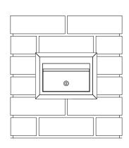
Complete remaining brickwork
